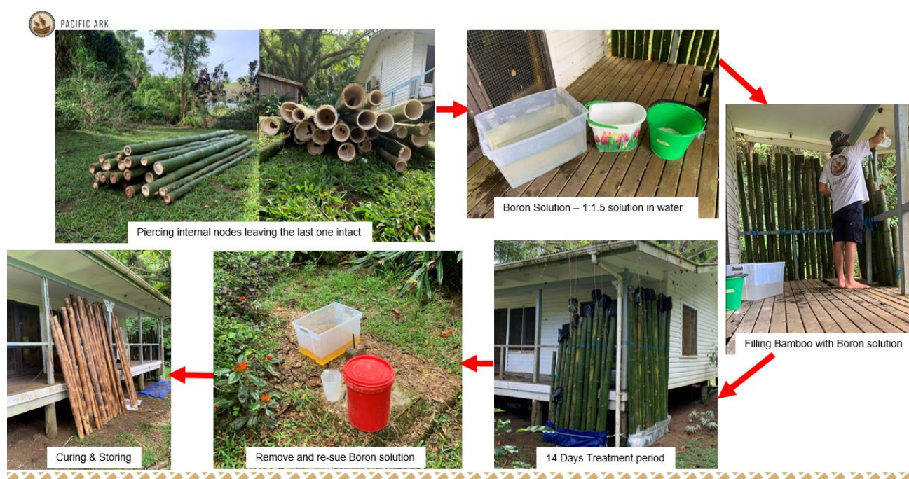
Figure 6-22: Vertical Soak Diffusion (VSD) setup for trials by Pacific Ark in Savusavu, Vanua Levu
