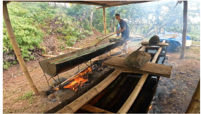
Figure 6-24: Placing bamboo into hot immersion tanks keeping it submerged at all times (Pacific Ark)
