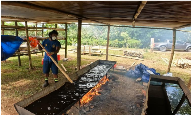
Figure 6-23: Dissolving boron mixture, prior to lacing bamboo into mixture (Pacific Ark)
