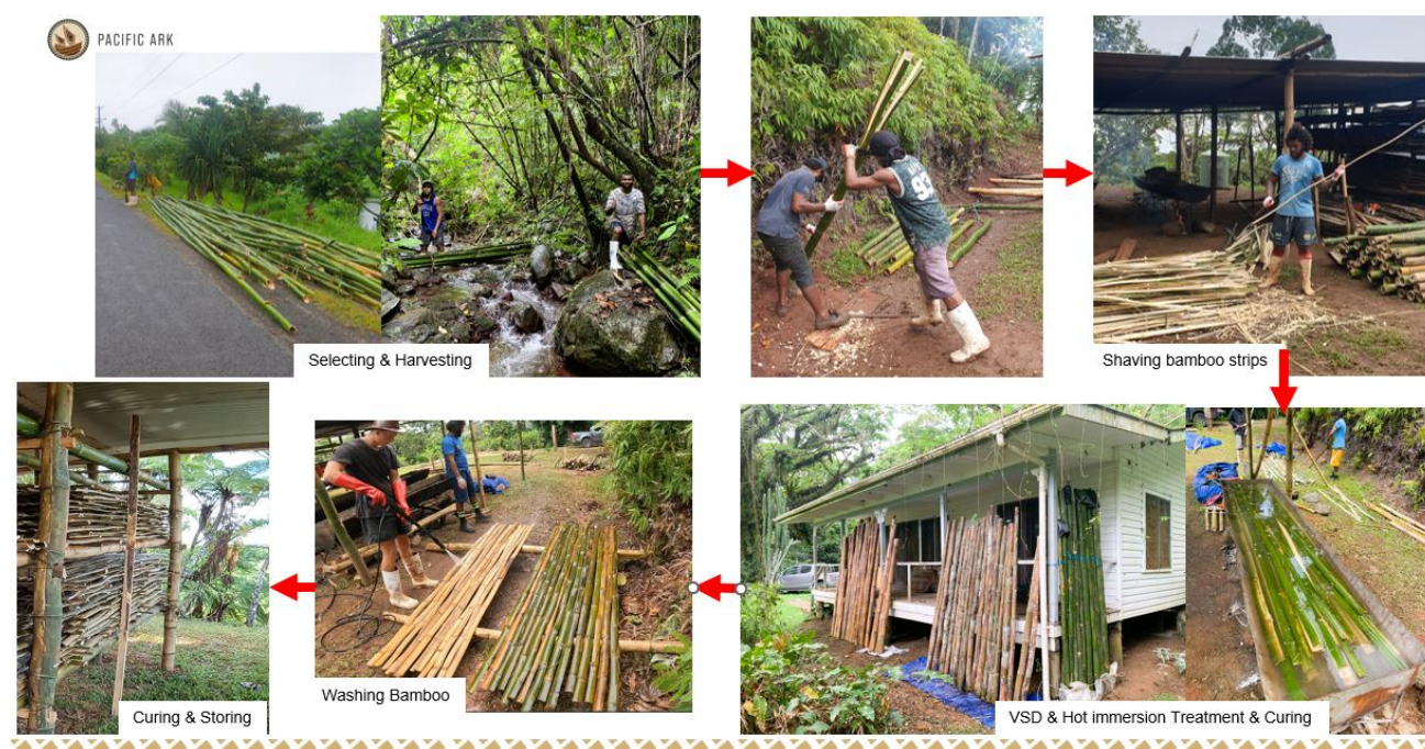
Figure 7-1: Pacific Ark trials from Bamboo Harvesting > Treatment > Prepping > Curing & storing
