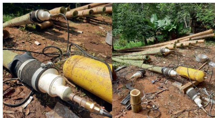
Figure 6-25: 1st trial of Modified Boucherie setup using portable low-pressure pump by Pacific Ark
